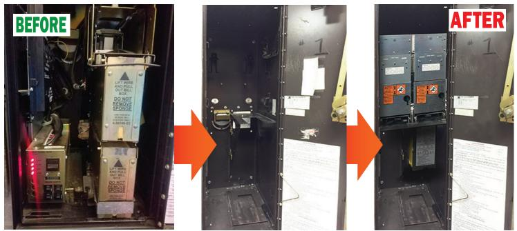
**Standard Change-Makers introduces a Modular Retrofit Kit for aging Rowe BC1400 change machines.** This is a unique solution, which allows you to remove all the internals of the installed machine and make room for two steel, Modular series coin hoppers AND one MEI downstacker bill acceptor with 500 bills stacker. The **BC1400 RETROFIT KIT** would give you a coin capacity of 6,400 Quarters and \$1-\$20 bill acceptance - all in EASY-TO-INSTALL assemblies.
