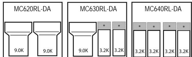
\* All 3.2K Hoppers can be upgraded to 5.2K Hopper capacity
